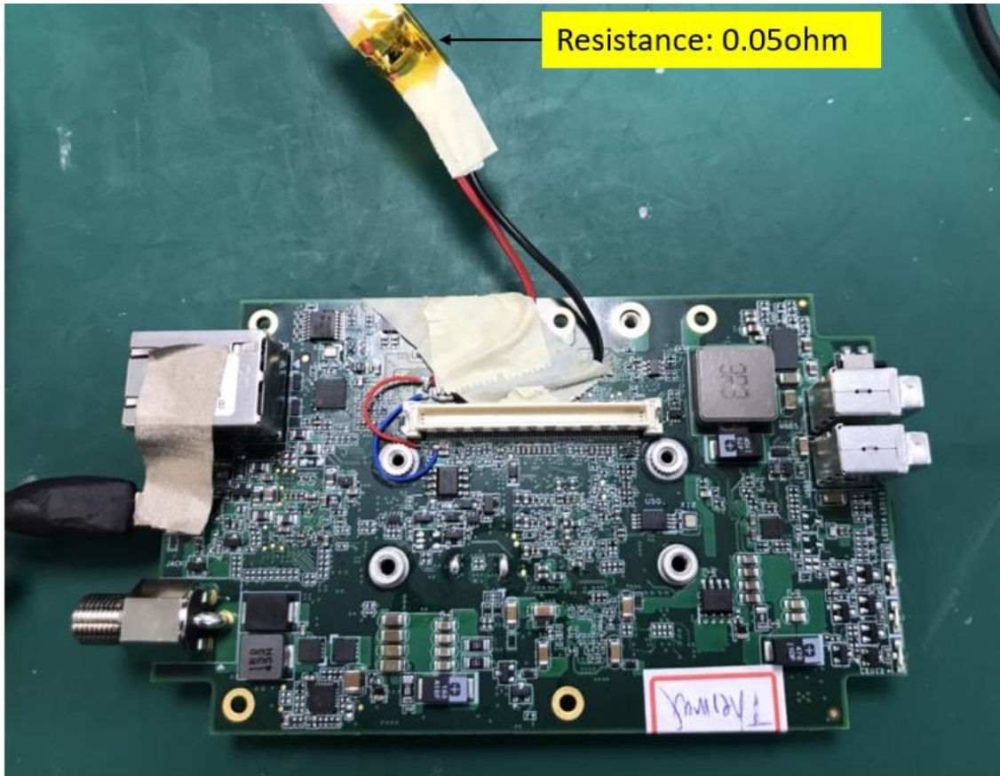
Welding the power wires on carrier board for measured ATS200 Power consumption
