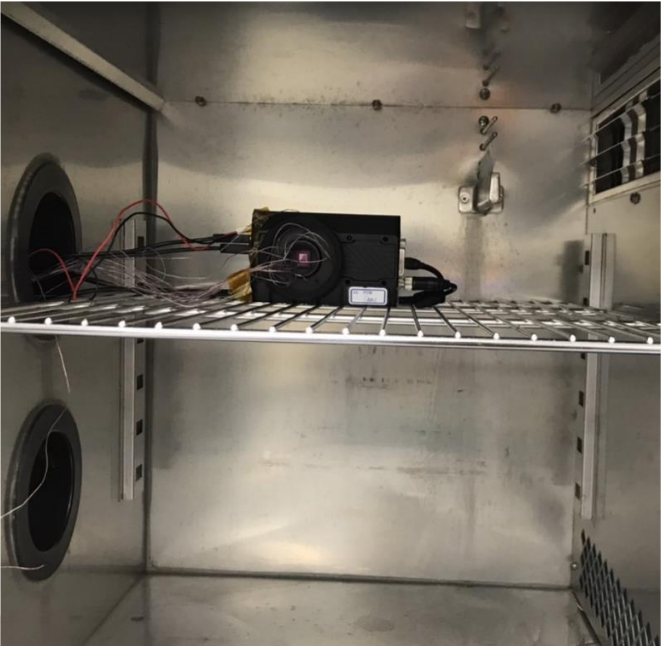
NEON-ATS200 thermal test in chamber
