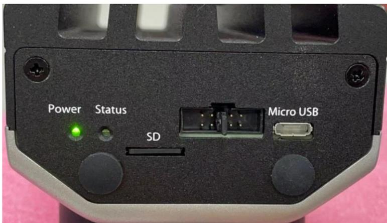
**Step 3-3:** Short pins 3 and 4 for two seconds (The Power LED will light out)
