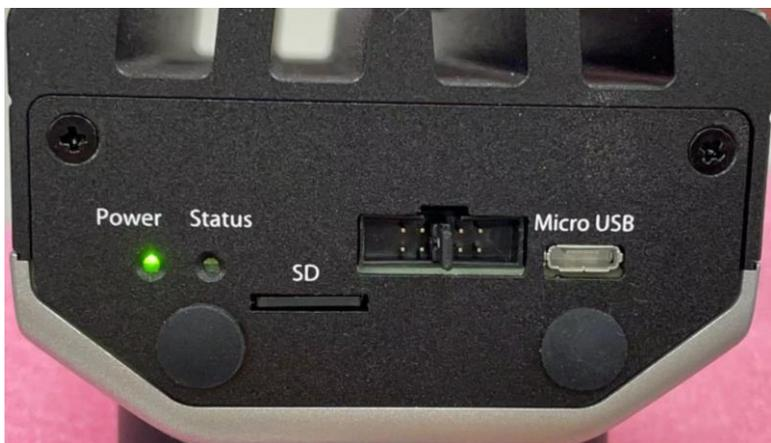
**Step 4-1:** Connect the NEON-2000-JNX to the **Host PC** with the Micro-USB to USB Type-A cable.
