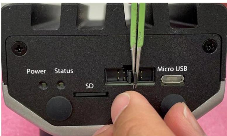
**Step 3-4:** Open pins 3 and 4. (The Power LED will light up)
